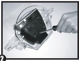
Secure the cradle to the Here<sub>2</sub>Anywhere unit with the Phillips head screw (Screwdriver not included.) Note: Screw goes through the large hole in the base.
