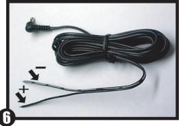
To connect the power use the included 10' power cable. Connect the finished end to the back of the cradle where it is marked "Power". Connect the bare wire end to the fused 12 volt DC from the display board.
