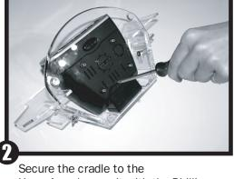
Here<sub>2</sub>Anywhere unit with the Phillips head screw (Screwdriver not included.) Note: Screw goes through the large hole in the base.
